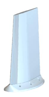
The 21-50-300 is vertically polarized, omni-directional antenna, compatible with all popular airborne radios operating within the 100 to 500 MHz frequency range. The antenna can handle 75 Watts of power and requires no external tuning.
