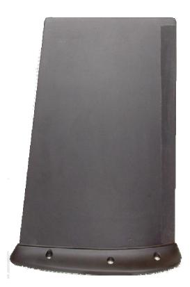
The 21-50-27-1 is a vertically polarized, omni-directional antenna, compatible with airborne radios operating within the 116 to 174 and 225 to 512 MHz frequency ranges. The antenna can handle 25 watts of power, requires no external tuning and is designed as a drop on replacement for AT1108/37R-2U types but having greater isolation between bands and better omni-directivity.
