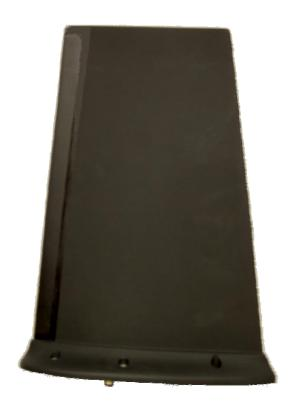
The 21-50-25 is a vertically polarized, omni-directional antenna, compatible with airborne radios operating within the 115 to 325 MHz frequency range. This antenna can handle 50 Watts of power and requires no external tuning.
