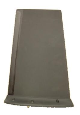
The 21-50-20 is a vertically polarized, omni-directional antenna, compatible with all popular airborne radios operating within the 30 to 400 MHZ frequency range. The 21-50-20 antenna can handle 50 Watts of power and requires no external tuning.
