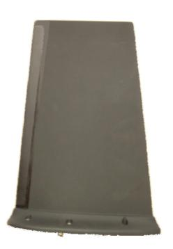
The 21-50-20-1 is a vertically polarized, omni-directional antenna, suitable for subsonic and supersonic aircraft, compatible with all popular airborne radios operating within the 30 to 400 MHZ frequency range. The 21-50-20-1 antenna can handle 50 Watts of power and requires no external tuning.
