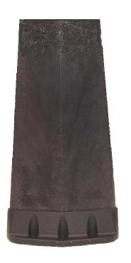
The 21-50-17 is a high performance combined UHF/L-Band airborne blade antenna suitable for helicopters and aircraft operating in excess of Mach 2.5
