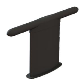
The 21-50-134 is a vertically polarized, omni-directional antenna, compatible with all popular airborne radios operating within the 66 to 530 MHZ frequency range. This antenna can handle up to 50 Watts of power and requires no external tuning.
