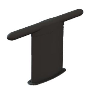
The 21-50-133 is a vertically polarized, omni-directional antenna, compatible with all popular airborne radios operating within the 30 to 512 MHZ frequency range. This antenna can handle up to 50 Watts of power and requires no external tuning.
