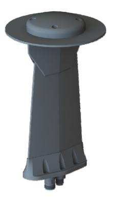
The 21-50-110-1 is a combination, vertically polarized VHF communications and circularly polarized active GPS antenna suitable for mounting on the upper surfaces of helicopters and sub sonic fixed wing aircraft.
