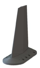
The 21-50-06-20 is a high performance combined UHF/L-band airborne blade antenna suitable for aircraft operating in excess of Mach 2. It is also ideal for use on aircraft subjected to rough-runway operation where both a protective leading edge strip and the solid aluminum alloy base block protect against debris impact.
