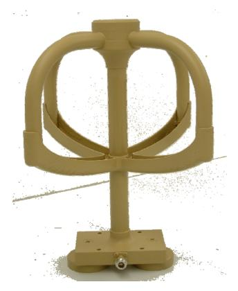
Satcom on-the-Move requires antenna pattern coverage to be as near to hemispherical as possible. The CAL 21-30-91MC07 utilizes a pair of quadrature connected UHF "droopy dipoles" with geometry arranged to maintain greater than 0 dBiC gain beyond a 120° cone.
