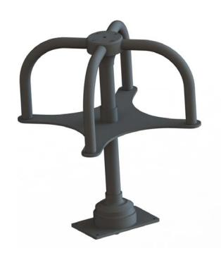
SATCOM on-the-move requires antenna pattern coverage to be as near to hemispherical as possible. The CAL 21-30-91 utilizes a pair of quadrature connected UHF "droopy dipoles" with geometry arranged to maintain greater than 0 dBiC gain beyond a 120° cone.
