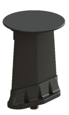
The 21-30-73 is a very low height receive only antenna covering VHF and UHF distress frequencies, VHF/FM maritime band and 890-960 MHz GSM frequencies. Design comprises a top loaded monopole with specially shaped radiating element to preserve patterns though the frequency range.
