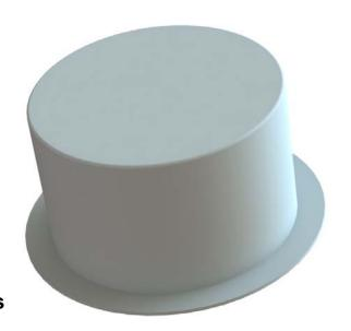
The 21-20-62 is a ruggedized VOR/Localiser/Glideslope antenna suitable for certain airborne and ground checking applications. For airborne use, the antenna can be mounted underneath an aircraft or helicopter fuselage where it can withstand ground and debris impact to a far greater extent than equivalent V-dipoles and other external antenna types. For ground use, the antenna provides a robust roof-mounted installation suitable for checking airfield VOR/ILS installations.
