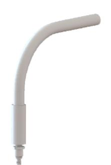
The 21-20-175 is a unique, wide band VHF antenna comprising a light gauge aluminum tube moulded into an insulator containing proprietary matching circuits producing an operating frequency of 118-165 MHz. This design is installed with a single hole skin cut out and secured from the inside with a 5/8 UNF nut. This antenna is DC grounded for lightning (LITS) and p-static protection.
