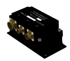
Military aircraft need to be able to depend on and maintain communications for broadband, frequency hopping V/UHF secure communications. In concert with Cooper Antennas range of tuneable antennas, the 21-171-15-2 digital Logic Converter Unit (LCU) receives frequency information from all versions of the ARC210, ARC231 or M3AR radio and tunes the antenna to the desired frequency which in turn optimizes the gain of the antenna.
