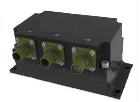
Military aircraft need to be able to depend on and maintain communications for broad-band, frequency hopping V/UHF secure communications. In concert with Cooper Antennas range of tuneable antennas, the 21-151-04 digital Logic Converter Unit (LCU) receives frequency information from all versions of the ARC210, M3AR and TRA6034C21 radios and tunes the antenna to the desired frequency which in turn optimizes the gain of the antenna.
