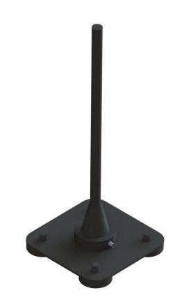
The 20-50-31 is a vertically polarized, omni-directional antenna designed for rapid deployment on steel roofs and shelters by incorporation of a strong magnetic mounting plate. This antenna has a relatively slim radiating element for low observability and has proprietary passive matching over the entire frequency band, thus requiring no external tuning.
