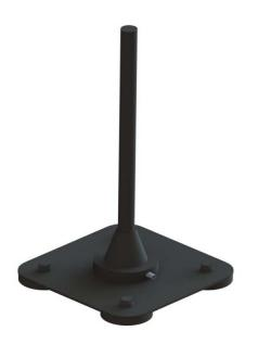
The 20-50-08 is a vertically polarized, omni-directional antenna designed for easy deployment on steel roofs and shelters by incorporation of a four point magnetic mounting plate. This antenna has a relatively slim radiating element and has proprietary passive matching over the two frequency bands, thus requiring no external tuning.
