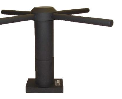
The 20-30-29VM and the 20-30-29VM/1 is a combined Hi-Lo angle UHF Satcom Antenna designed for installation on military vehicle roof, shelter or housing via a 4 hole mounting plate. The only difference between 20-30-29VM and the 20-30-29VM/1 is that in the 20-30-29VM the coaxial connectors are fitted to the bottom of the antenna base and in the 20-30-29VM/1 they are fitted to the side of the base.
