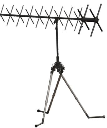
The 20-30-19 is a right hand circularly polarized quick-erect antenna designed for a wide range of special operational requirements. As a free-standing tripod mounted device it provides +13 dBiC gain and can be "pointed" in any angle thru a solid 180° to align with the satellite.
