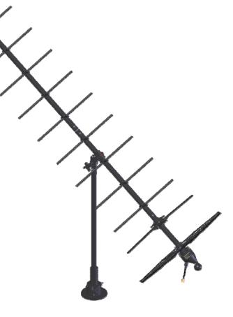
The 20-30-17 is a right hand circularly polarized quick-erect antenna designed for a wide range of special operational requirements. As a free-standing tripod mounted device it provides up to +14 dBiC gain and can be "pointed" in any angle thru a solid 180° to align with the satellite. It can also be hard mounted for vehicular, shelter or fixed shipborne use.
